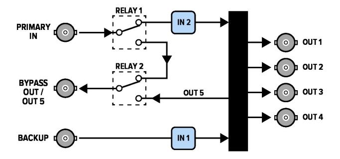
The R2-6002-DA-1X4-12G-B with Bypass Relay diagram illustrates how the bypass relay system functions within the distribution amplifier. This system provides redundancy and automatic signal switching to ensure uninterrupted video distribution in case of power failure.
