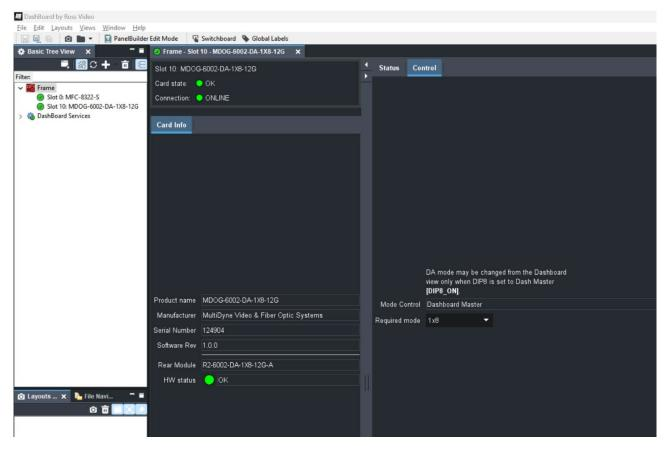
In the **Card Info tab**, users can change the mode and view the product information, such as serial number, software version, and hardware status. The module mode may only be changed from the DashBoard view when DIP8 is set to Dash Master (DIP8\_ON).
