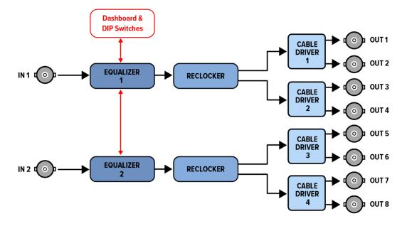
The **MDoG-6002 Block Diagram** provides a visual overview of the internal signal flow and key components that process the SDI signals within the distribution amplifier.
